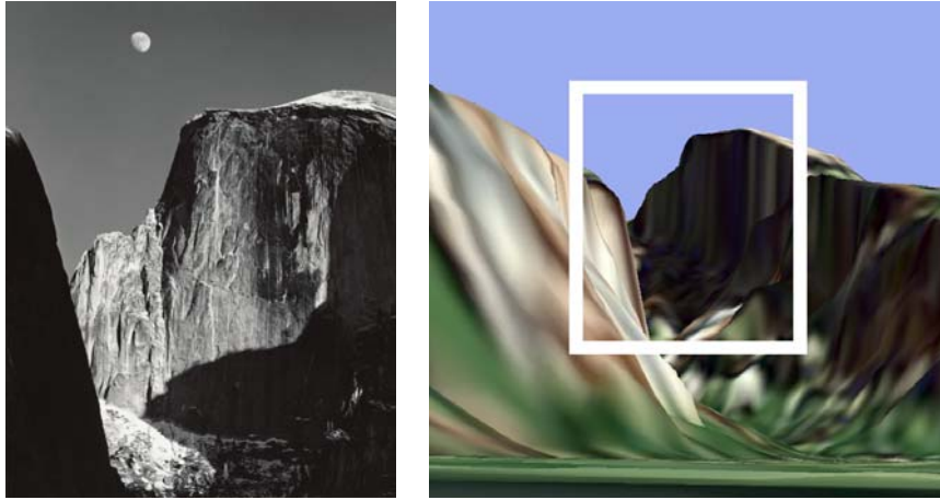
Figure 5.8: A registered historical photo. Left: Moon and Half Dome , 1960. Photograph by Ansel Adams. This historical photo taken by Ansel Adams was automatically registered to our Half Dome reconstruction. Right: rendering of DEM data for Half Dome from where Ansel Adams was standing, as estimated by the system. The white border was drawn manually for clarity. (DEM and color texture courtesy of the U.S. Geological Survey.)
