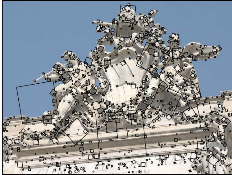
Figure 3.3: Example set of detected SIFT features. Each detected SIFT feature is displayed as a black box centered on the detect feature location. SIFT detects a canonical scale and orientation for each feature, depicted by scaling and rotating each box.
