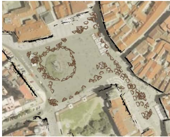
Figure 3.9: Example registration of cameras to an overhead map. Here, the cameras and recovered line segments from the Prague data set are shown superimposed on an aerial image. (Aerial image shown here and in Figure 5.1 courtesy of Gefos, a.s. [51] and Atlas.cz.)
