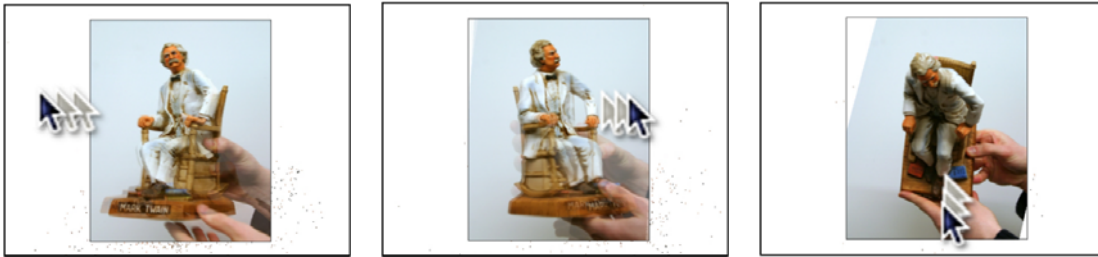
Figure 6.9: Orbiting a home-made object movie of Mark Twain. This sequence shows screenshots from a interaction session with a figurine of Mark Twain. The input images are from a video taken of the figurine while rotating it around in front of the camera. The images show a user clicking and dragging the mouse to rotate the object to the right (right image), left (middle image), and down (left image).
