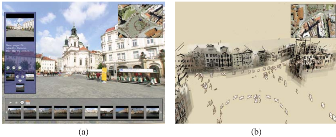
Figure 5.1: Screenshots from the Photo Tourism viewer. Left: when the user visits a photo, that photo appears at full-resolution, and information about it appears in a pane on the left. Results of search operations appear in the thumbnail pane on the bottom of the screen, and an overhead map is shown on the upper-right side of the screen. Right: a view looking down on the Prague dataset, rendered in a non-photorealistic style.
