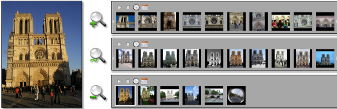
Figure 5.5: Zooming controls . Left: an image from the Notre Dame data set. Right: the results of searching for details (top), similar images (middle), and zoom-outs (bottom), starting from this input image.
