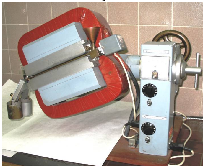
Fig. 8.10. Operating principle of the Frantz isodynamic separator (IDS) (after Svoboda, 1987 with modifications) (a) and its photograph (b)
