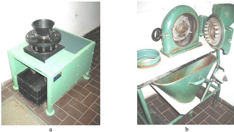
Fig. 3.17. Laboratory cone crusher (a) and laboratory finger disintegrator (b)
