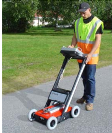
Plate D1 Ground Probing Radar (Courtesy of Radiolocation Ltd.)
