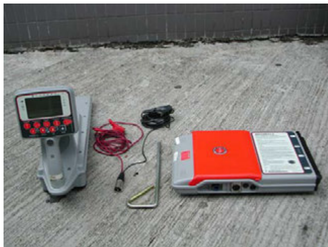
Plate C2 Components of Electromagnetic Type Detection Equipment
