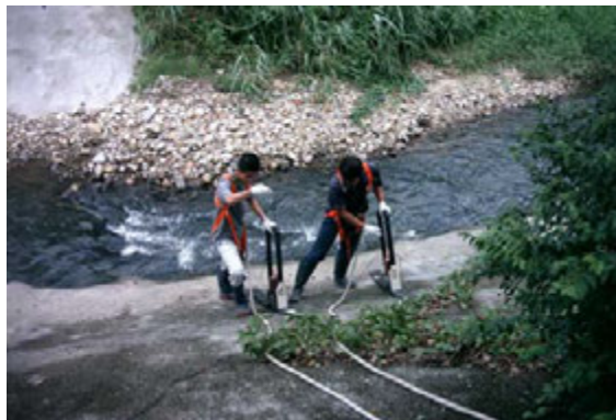
Plate D2 Ground Probing Radar on Slope (Courtesy of the Hong Kong Institute of Utility Surveyors)
