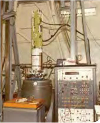
2-20 : The integrity of the flight control unit being examined by testing to ensure that it functioned while being subjected to severe vibration levels at the GAF Environmental Testing Laboratory.
