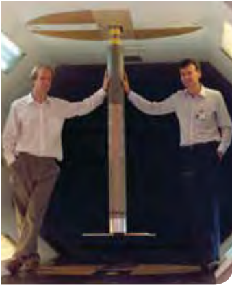
6-14 : Ian Mitchelhill (ASTA) and Leon MacLaren (seconded from the Aeronautical Research Laboratory to AWA) seen here with the Pressure Air Data Assembly fitted to a decoy in the low speed wind tunnel at ARL. These were the final tests to establish the performance of the assembly prior to flight tests. Ice shapes are visible as a pink patch on the decoy for these tests.
