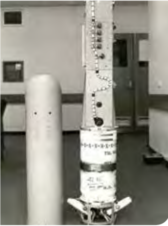
2-14 : The shortening of the Murawa sustainer motor is clear from the weld to the motor case. The use of this motor allowed the use of many existing components for the flight control system.
