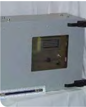
8-6 : The Fire Control Panel.
