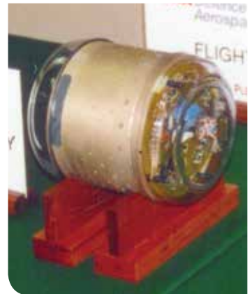
6-12 : Pressure Air Data Assembly.
