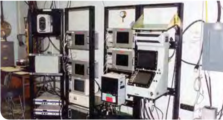
8-18 : The Active Missile Decoy suite of shipboard decoy firing and control equipment with instrumentation is set to work at Woomera for final functional testing prior to tests on ship.
