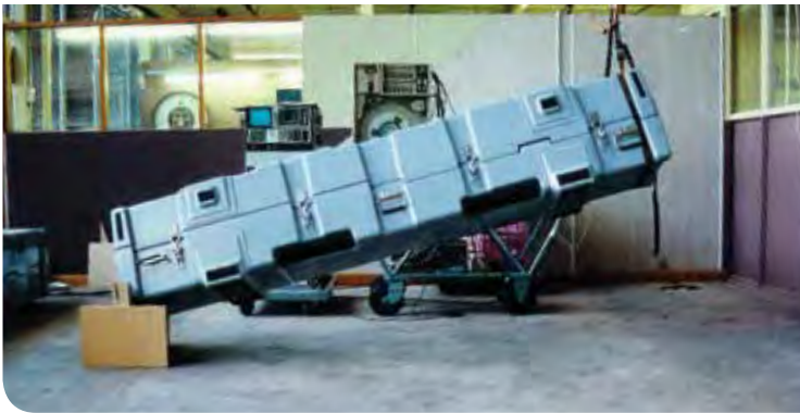
6-30C : Surviving the corner drop test was mandatory.
