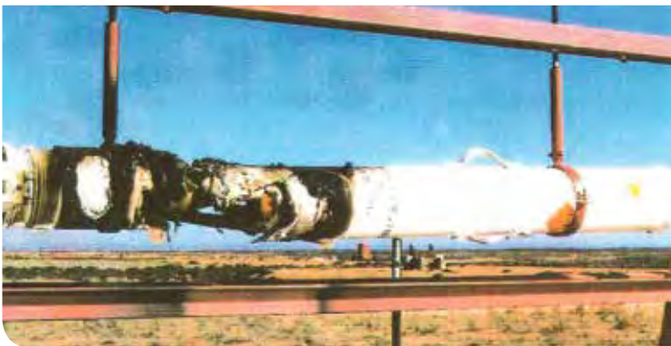
6-30D : 20 mm bullet Impact Test Rocket Motor Assembly.
