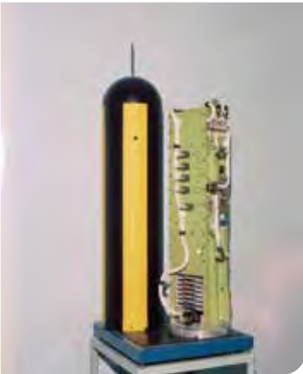
2-15 : The completed flight control system showing electronics and top cover to the vehicle.
