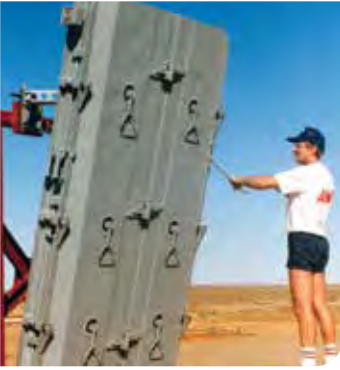
6-17 : Ian Jolley of AWA operating the simple scissor mechanism to cause the launcher to tilt from vertical stowed position for launching.
