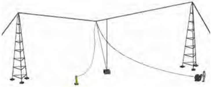
2-23 : The 'Hoveroc' tethered test used two large towers at Port Wakefield Proof Range, South Australia.
