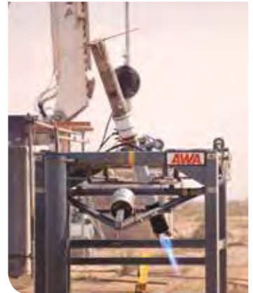
6-23 : Gimbal Firing Test DT-IIA Phase 1 at Woomera.
