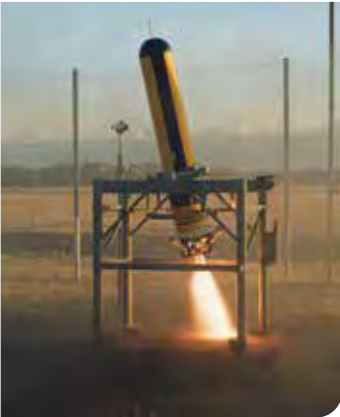
2-21 : The 'Hoveroc' test vehicle being tested while being allowed to rotate in a set of gimbals. The tests of the Winnin thrust vectoring system were successfully completed in October 1980.
