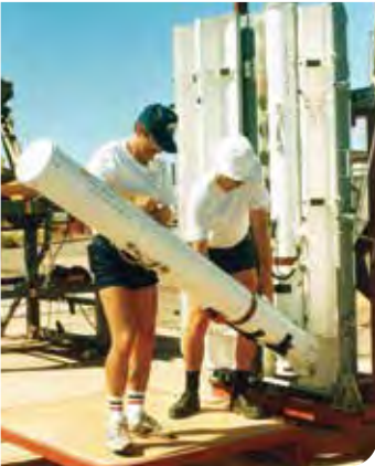
6-18 : Loading a decoy canister into a launcher was exercised many times during flight trials on land and later on board ship, and then later during training courses for Navy personnel.
