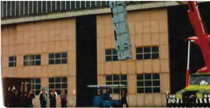
6-30B : Establishing susceptibility to damage by dropping the decoy in a shipping container from 12 metres.
