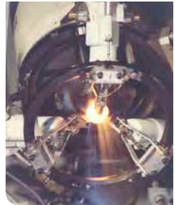
2-19 : The thrust control system and the modified Murawa rocket motor under test.
