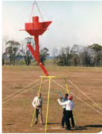
4-8 : The team guiding the captive carry unit into first docking rig.
