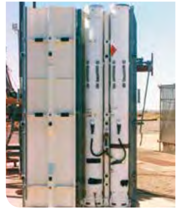
6-15 : Two decoy canisters are shown fitted to the launcher before the launcher doors are closed.
