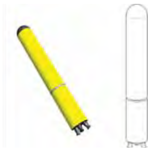
2-7 : Sketch of the 'Directly Supported Rocket' vehicle. One of several ideas preceding the 'Hovering Rocket' was a large conventional rocket motor with multiple nozzles. The thrust was to be varied in the secondary nozzles.
