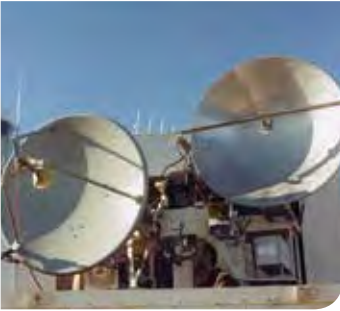
4-15 : Telemetry and simulator antennas received data from the payload and Captive Carry Unit and a simulator represented the missile.
