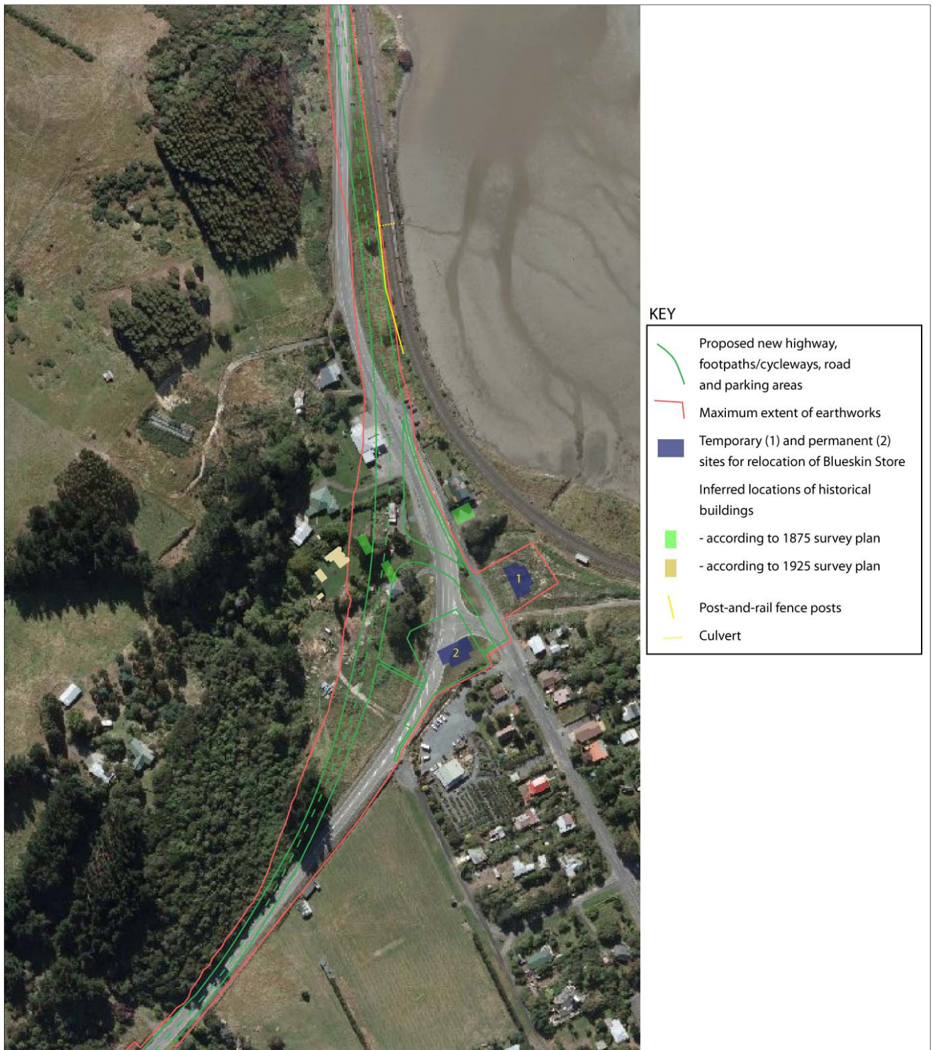
Figure 8. Proposed realignment of SH1 at Waitati showing maximum extent of earthworks in relation to inferred locations of possible archaeological sites.
