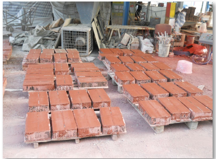
Paver blocks made of cement-stabilised marine mud
