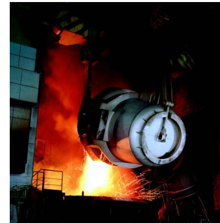
Chargieren von Flüssigstahl in einem Elektroofen in Edelstahlwerk Shanghai Baosteel No. 1 Source: SMS group Charging of liquid steel into an electric arc furnace at the stainless steel meltshop of Shanghai Baosteel No. 1
