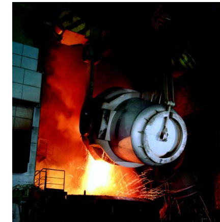
Chargieren von Flüssigstahl in einem Elektroofen in Edelstahlwerk Shanghai Baosteel No. 1 Source: SMS group Charging of liquid steel into an electric arc furnace at the stainless steel melthop of Shanghai Baosteel No. 1
