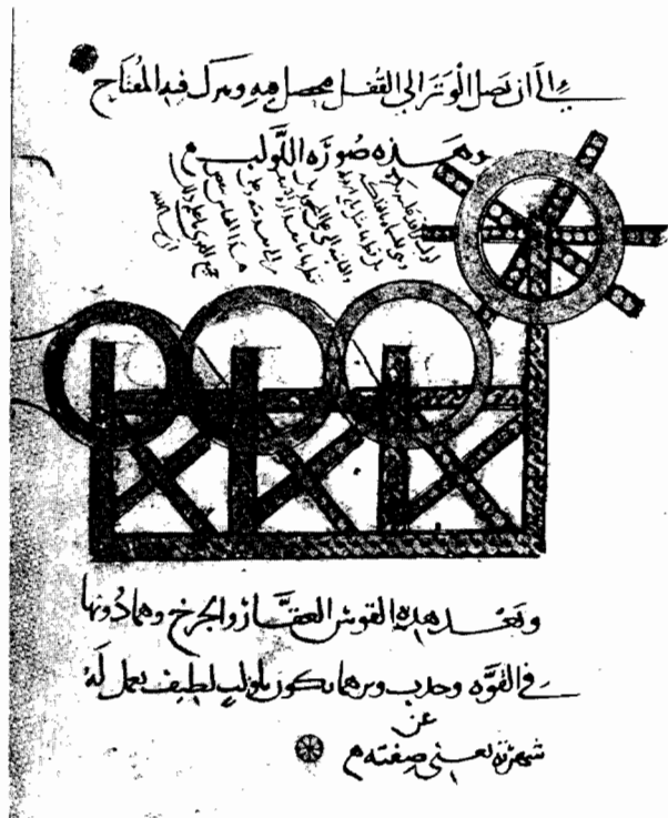
The ziyar and its loading mechanism. This was a large mounted crossbow reinforced by a wooden frame with taut ropes giving added strength to the arms of the bow. The bolt emerged from a small 'gateway' in the centre of the weapon. From al Tarsusi's late 12th-century military treatise (Ms. Hunt. 264, Bodleian Lib., Oxford) See Plate C1.
