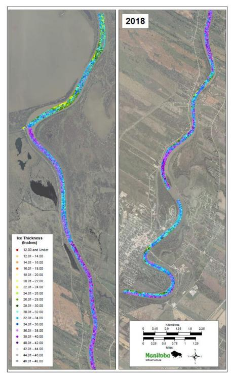
Figure 6 – Ice Thickness Measurements based on Ground Penetrating Radar, Lower Red River
