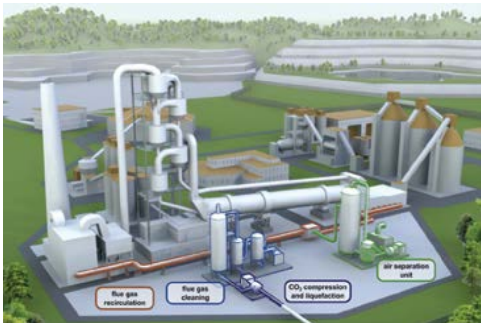
Figure 4: Oxyfuel CCS as applied to a cement plant
