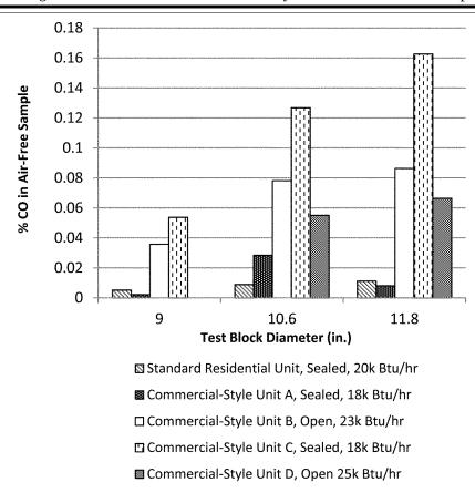
Figure III.4 CO Emissions by Test Block Diameter
