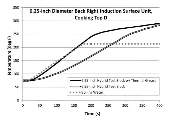
Figure III.2 Effect of Thermal Grease on Initial Test Block Temperature Rise
