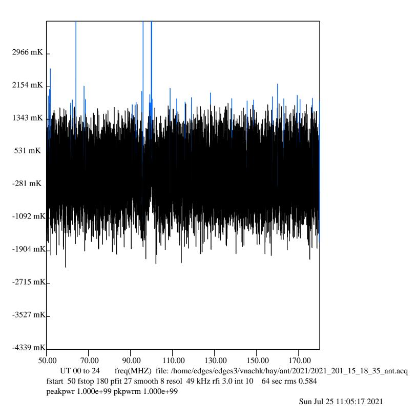
Figure 5. 3 Position switched power with RFI excision with only one signal at 100 MHz at 81 dBm
