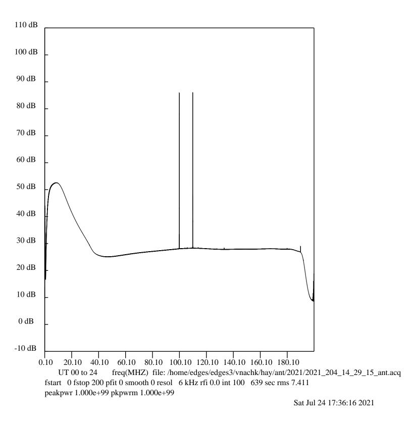
Figure 1. Antenna spectrum with -81 dBm signals from RF explorer signal generators at 100 and 110 MHz
