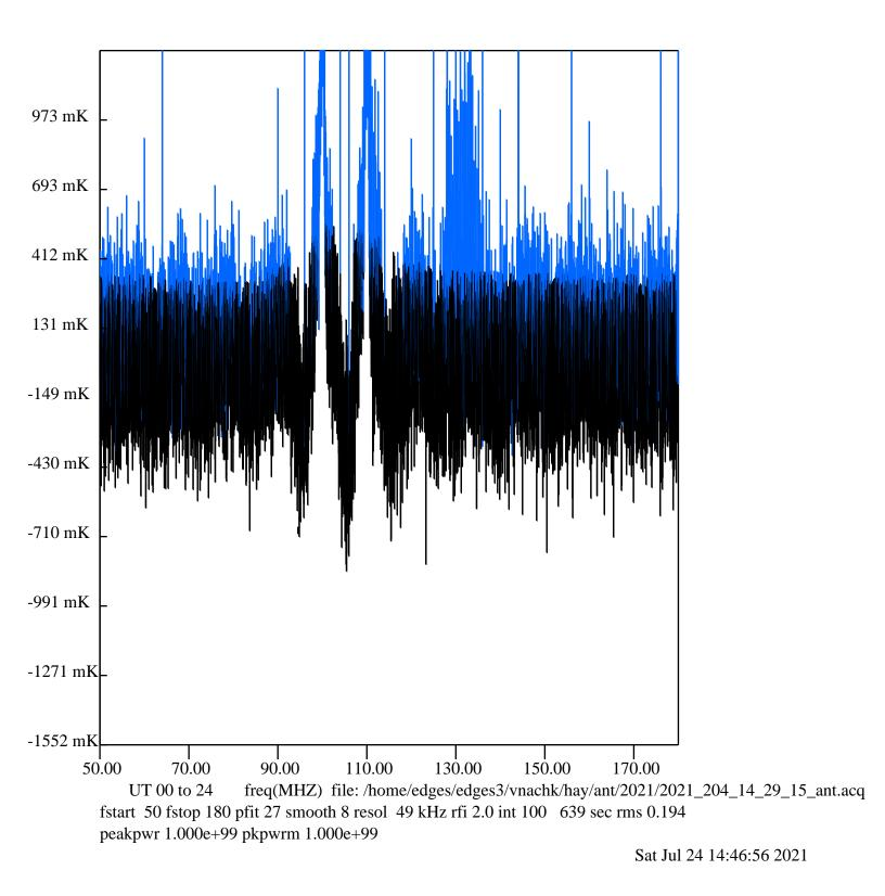
Figure 4. 3 Position switched power with RFI excision when both signals at 81 dBm.
