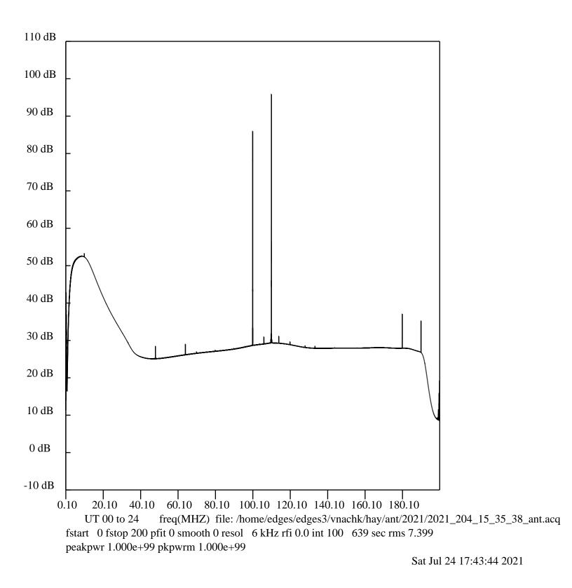
Figure 3. Power level of 110 MHz increased to -71 dBm at which point the ADC is saturating.
