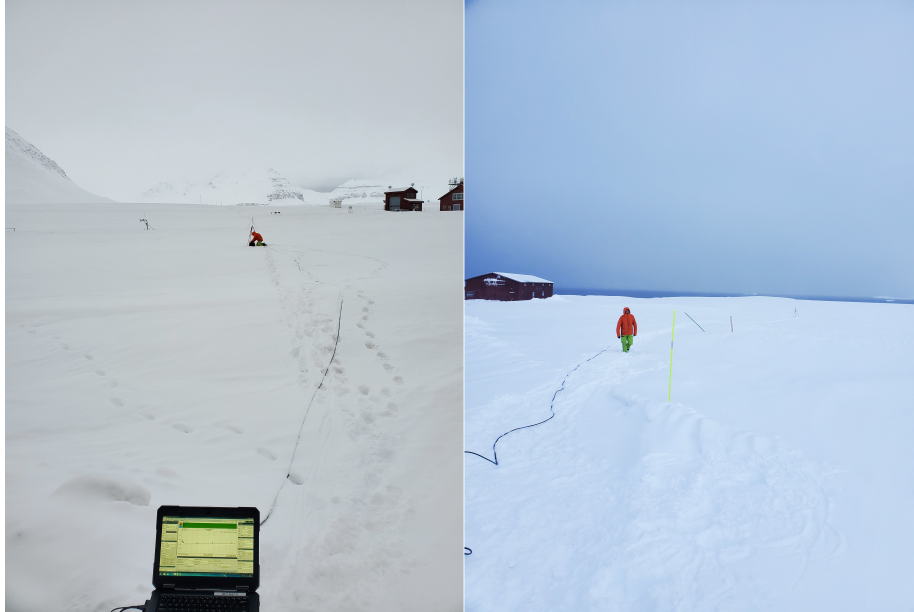
Figure 6: Example test setup for measurements inside the Ny Ålesund settlement, near the miniature steam train. The picture on the right is the location that showed the least amount of interference within the town site.
