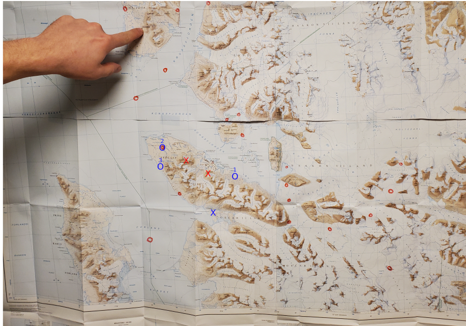
Figure 11: Locations with radio communication on the 170 MHz communication frequency. The red 'X' denote locations of the 170 MHz repeater stations. The blue 'O' denote the locations of the tests made outside the townsite. The red 'o' show the locations where communications have been made on the 170 MHz radio band in the field. The blue 'X' shows a potential promising location for the receiver. A local of Ny Ålesund has stated that there is no radio reception there. Pictures of this "sandbar" area are provided in section 4.3.1.
