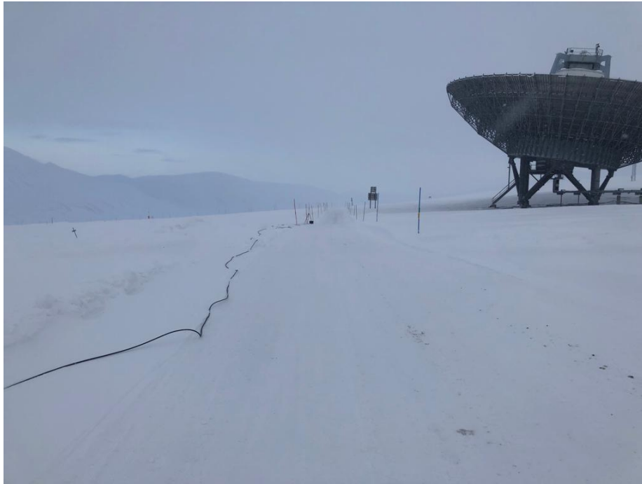
Figure 4: Picture of setup at Svalbard EISCAT. The large antenna on the right was not transmitting at the time of experiment. The center frequency for this radar is 500 MHz.
