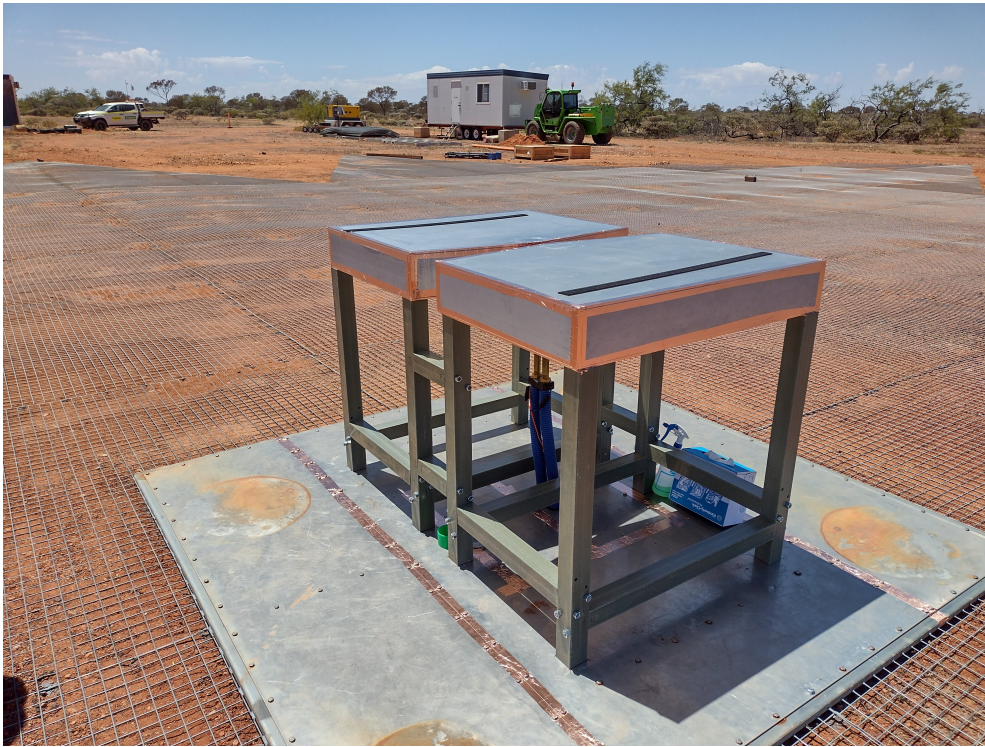
Figure 7: Copper tape applied to seams of antenna and base-plate.
