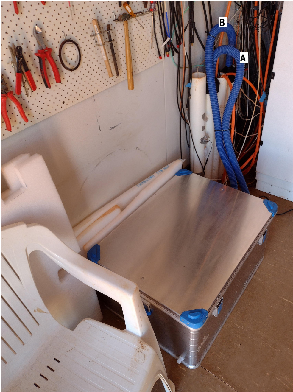
Figure 11: The EDGES-3 air circulation box.
