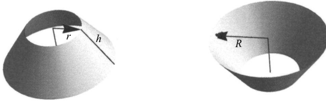
Figure 14.1. Left: Frustum of a cone of slant height h and upper radius r . Right: Same frustum, turned upside down to exhibit the lower radius R .
