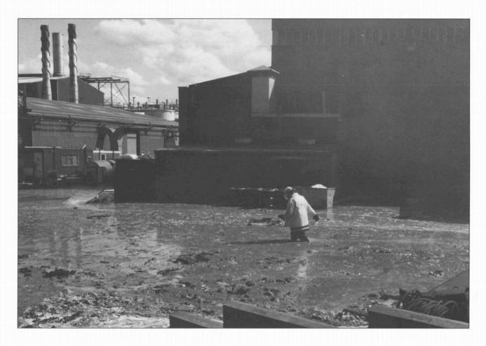
*Figure 13:* Sludge-like mixture from fire-fighting water and materials from the fire affected areas which flowed downhill to the centre of the site and beyond. Courtesy of West Yorkshire Fire Service.
