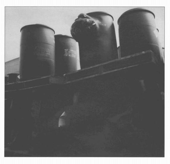
Figure 8: Plastic drums on the fire block flammable liquid storage area showing heat radiation damage and effects of pressurisation.
