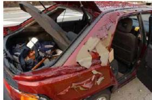
Figure 6 Damaged car 170 m away from the crater of the Ghislenghien accident
