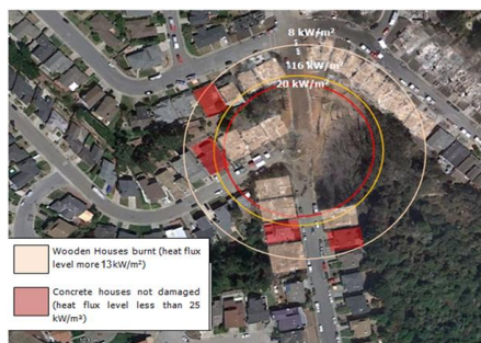
Figure 13 Heat flux distances according to damages during the San Bruno accident 2010
