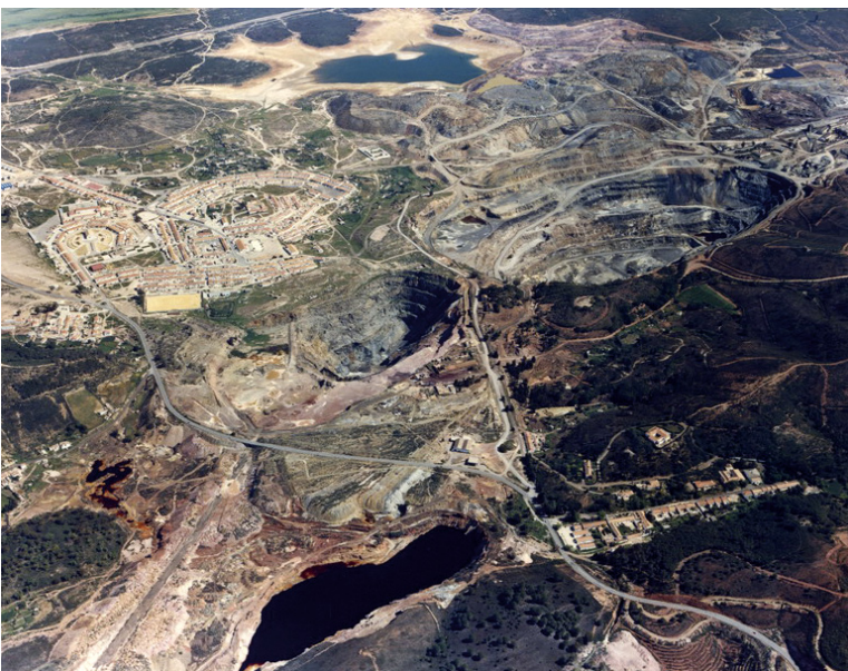
Figure 9. Aerial view of the works in Tharsis. The open pit in the lower margin is the Southern Vein, and the flooded one to the right is the Central vein. The big pits of Sierra Bullones and Northern Vein are in the Northern Vein.
