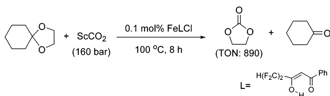
Scheme 21. Synthesis of a Cyclic Carbonate from a Cyclic Ketal
