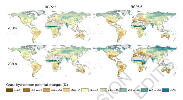
Figure 6.20 Global spatial patterns of changes in gross hydropower potential based on climate forcing from five climate models. Changes are shown for the 2050s (upper) and the 2080s (lower) for the low emission scenario (RCP2.6; left) and highest emission scenario (RCP8.5; right) scenarios relative to the control period (1971–2000). [Data source: (van Vliet et al. 2016a)].
