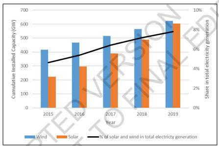
Figure 6.6 Global solar and wind electricity installed capacities (GW) from 2015–2019 and their combined share in total electricity generation Source: data from (IEA 2021a) IRENA, 2021).
