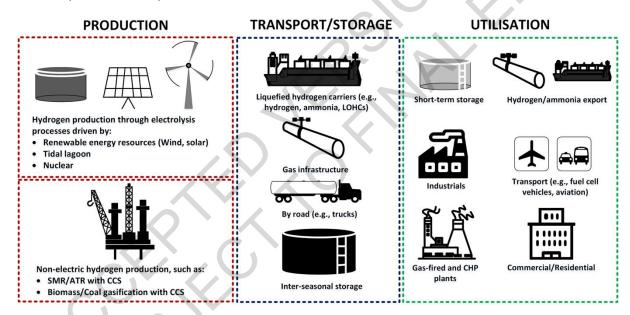
Figure 6.17 Hydrogen value chain. Hydrogen can be produced by various means and input and fuel sources. These processes have different emissions implications. Hydrogen can be transported by various means and in various forms, and it can be stored in bulk for longer-term use. It also has multiple potential end uses. CHP: Combined heat and power
