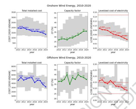
Figure 6.11 Global weighted average total installed costs, capacity factors, and LCOE for onshore (top) and offshore (bottom) wind power of existing power plants per year (2010-2020). The shaded area represents the 5th and 95th percentiles and the red dashed line represents the fossil fuel cost range.
