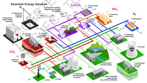
Figure 6.23 Schematic of net zero emissions energy system, including methods to address difficult-toelectrify sectors. (Source: Davis et al. 2018)
