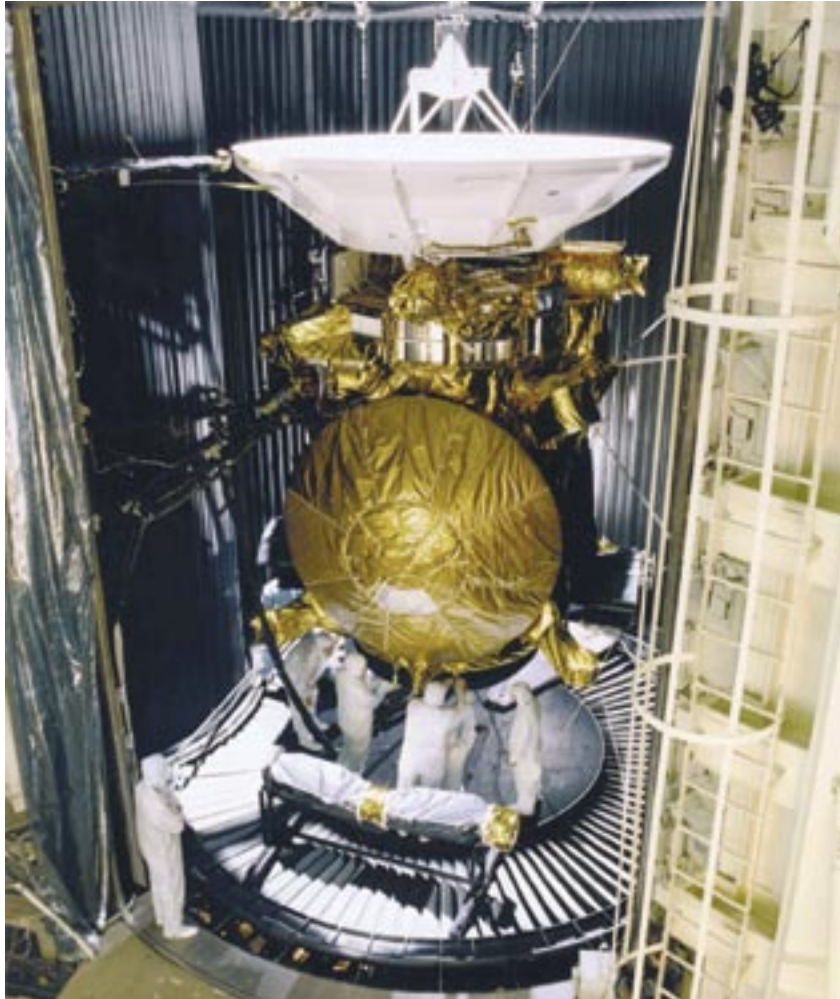
Figure 4: The Huygens probe (centre) is mated to the large body of the Cassini spacecraft. (Credits: NASA)
