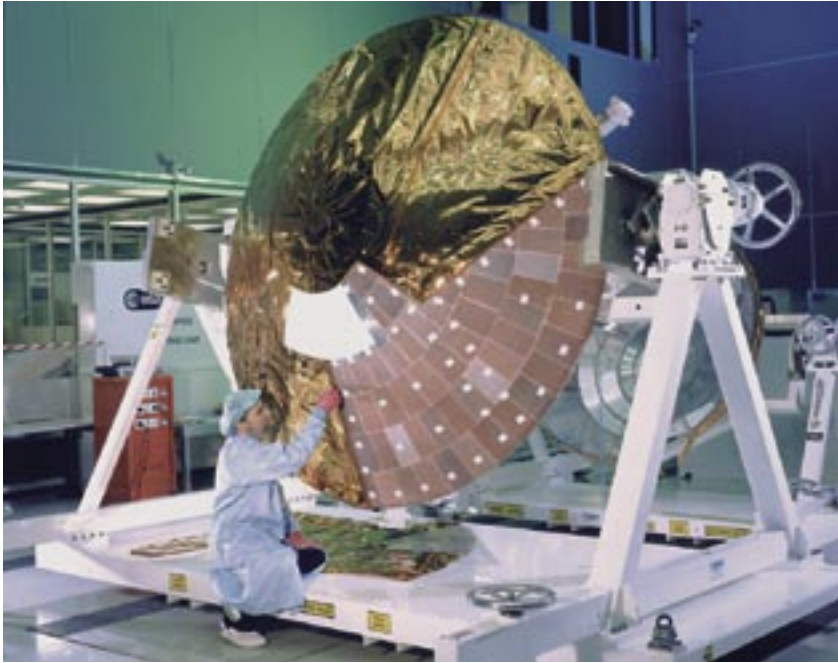
Figure 5: Installation of the Multi-Layer Insulation (MLI) blankets on Huygens' front shield and back cover. The intense aerodynamic heating during entry rapidly vaporised the MLI, and the 20 mm thick sponge-textured brown tiles insulated the carbon fibre internal structure and the descent module from the intense radiation of the hypersonic shock wave.
