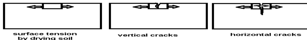
Figure 8: shows Progression of desiccation or shrinkage cracks
