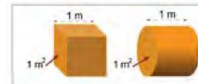
of unit length and unit cross section, i.e. 1 cubic metre. (In practice this would be virtually impossible to measure directly.) The resistivity of copper is  $1.68 \times 10^{-8} \Omega \text{ m}$ .
