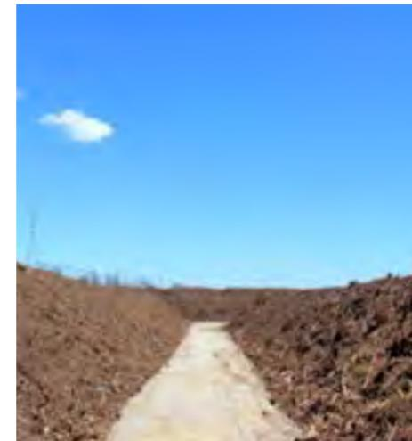
**F**igure 6: An Industrial composting facility (left) and a home compost (right). The temperature of an industrial compost heap will reach over 60°C while a home compost will typically reach less than 50°C. Commercial compost heaps are managed to maintain temperature, moisture and aeration making them much more efficient at decomposing organic matter (including biodegradable plastics) than home compost heaps
