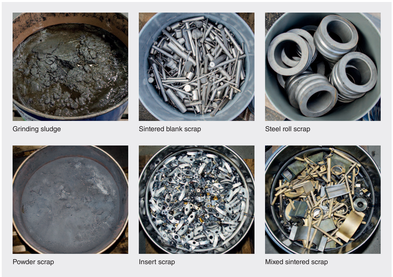
Figure 2: Examples of tungsten carbide new scrap, also called primary or production scrap. Scrap generated during manufacturing of tungsten products. Courtesy of Wolfram Bergbau und Huetten AG
