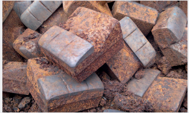
Figure 5: Collected old scrap stemming from end-use in mining and construction. The tools consist of cemented carbide and steel. They are stored for dismantling and cemented carbide separation. Courtesy of M Sicho, GTS - Global Tungsten Solution s.r.o., Czech Republic
