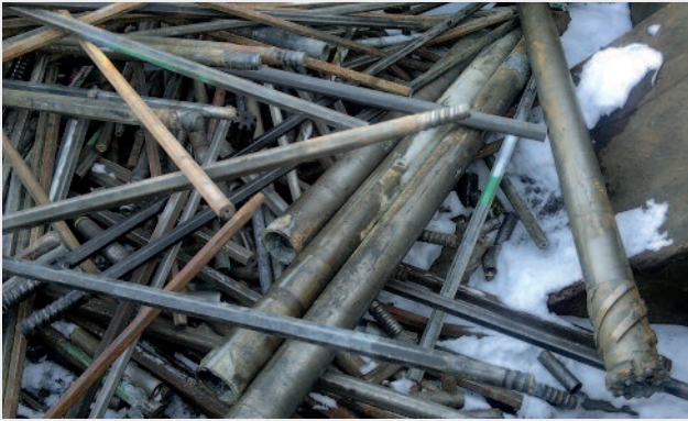
Figure 5: Collected old scrap stemming from end-use in mining and construction. The tools consist of cemented carbide and steel. They are stored for dismantling and cemented carbide separation. Courtesy of M Sicho, GTS - Global Tungsten Solution s.r.o., Czech Republic
