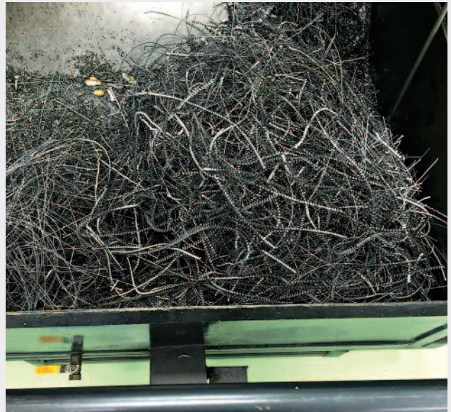
Figure 6: Tungsten high-speed steel (HSS) scrap, blanks and turnings, as collected by the toolmaker (new scrap) for recycling in an HSS smelter. Courtesy of W D Schubert
