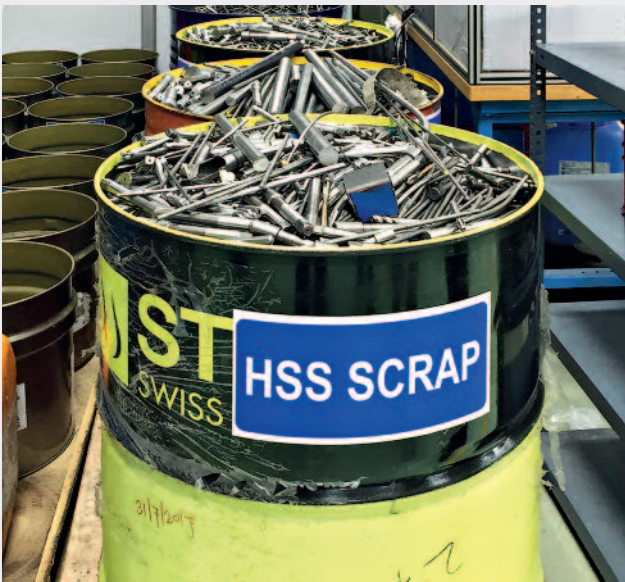
Figure 6: Tungsten high-speed steel (HSS) scrap, blanks and turnings, as collected by the toolmaker (new scrap) for recycling in an HSS smelter. Courtesy of W D Schubert
