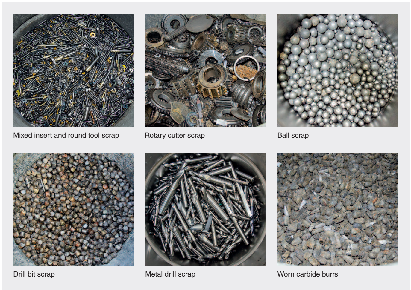
Figure 1: Examples of cemented carbide old scrap. Tungsten products after their end-of-life. Courtesy of Wolfram Bergbau und Huetten AG
