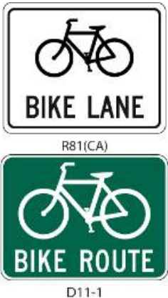
Figure 2-3: Caltrans Bikeway Signs
