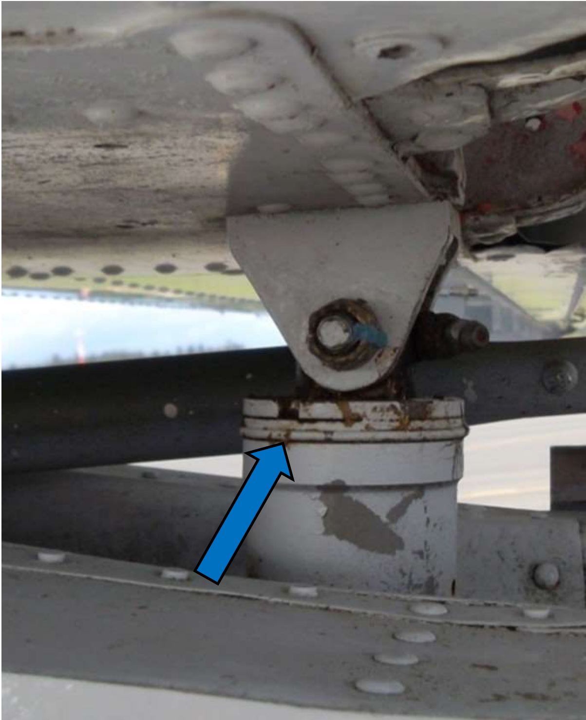
Figure 2 – Stabilizer Actuator – Upper Attachment to Stabilizer (External)
