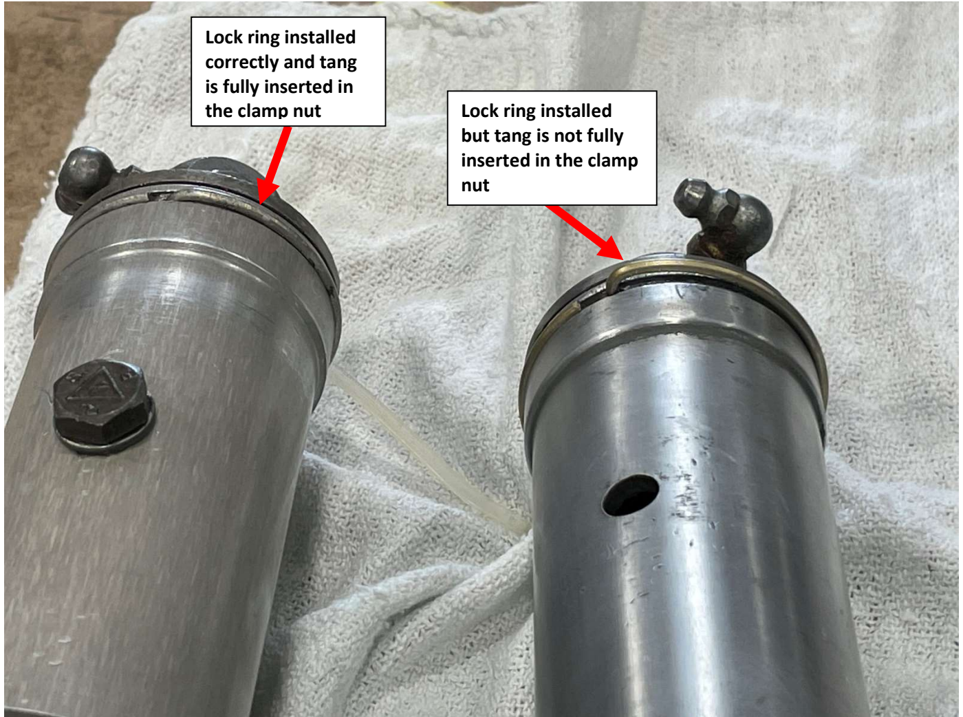
Figure 3 – Correct and Incorrect Installation of Lock Ring
