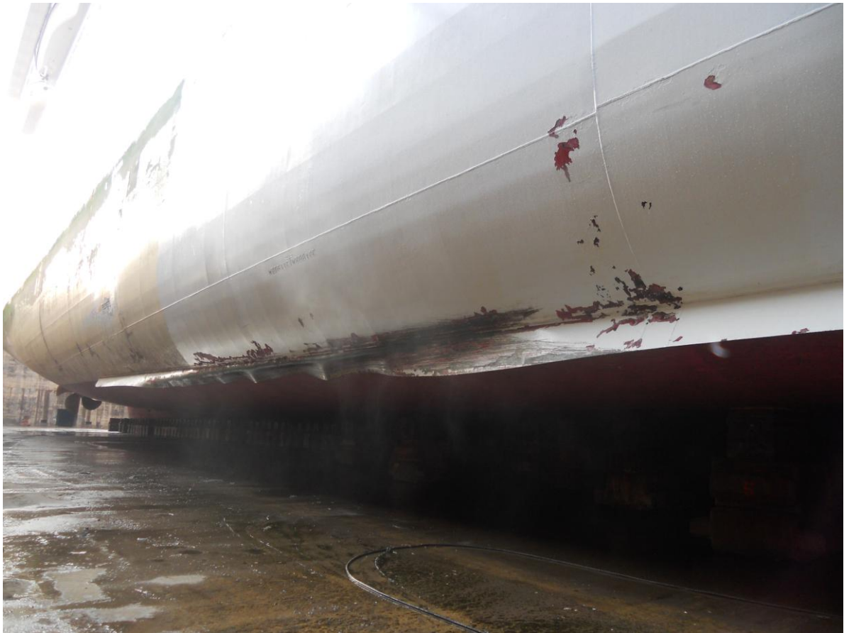
Following pictures show the hull area interested by the contact (taken from sister ship Costa Serena):
