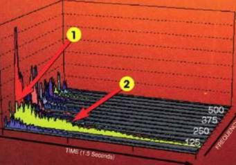
FT: These graphs are Fast Fourier Transforms. In simple terms, a ourier transform can illustrate, at the same time, the amount of all requencies produced by a resonating element. Time is epresented by what is moving forward at you. Frequency is shown by low end on the left and high end on the right. And the amount of any frequency is represented by its height.
