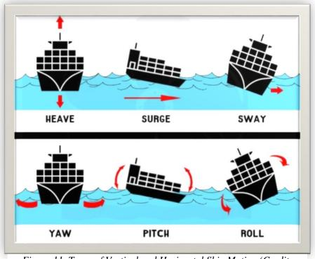
Figure 11. Types of Vertical and Horizontal Ship Motion (Credit: Thomas Smith Shipping)
