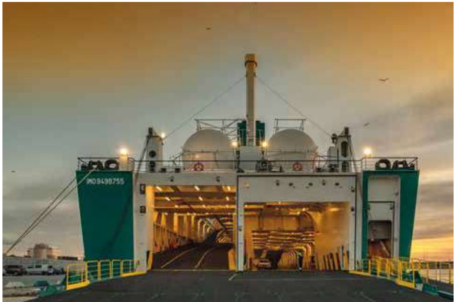
Access on the portside to the upper deck and on the starboard side into the main deck.
