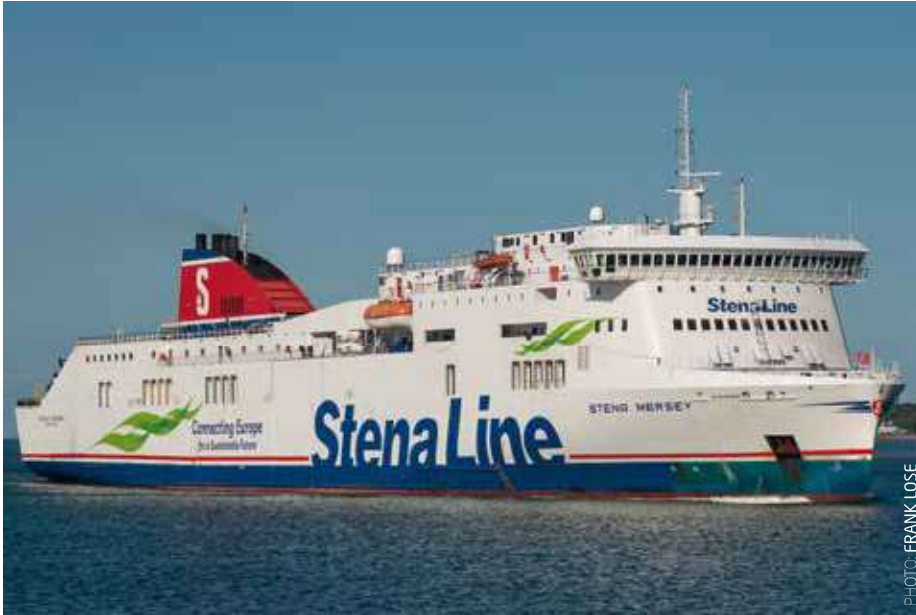
STENA MERSEY and STENA LAGAN will be lengthened by 36m. The ship's bows will be modified to allow for double-deck drive-through loading.
