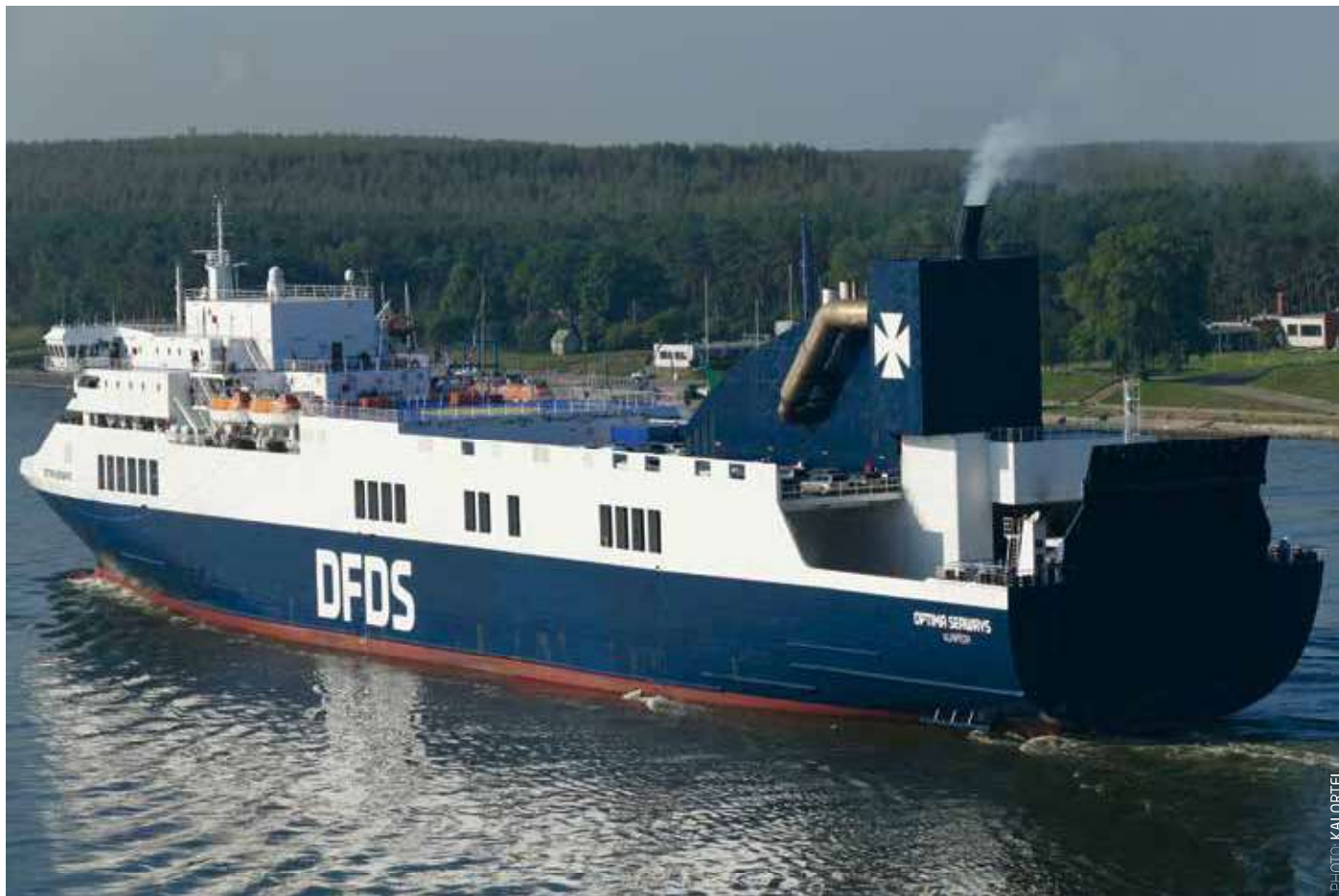
The 1999-built OPTIMA SEAWAYS is an early-generation Visentini ro-pax. A scrubber has been retrofitted to comply with the SECA rules in the Baltic Sea.
