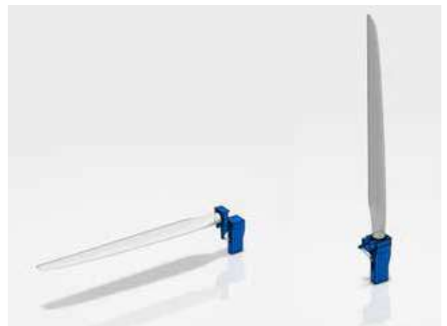
The shape of things to come? NAOS's Wing Sail Module is a modular concept, the blades of which can fold down.
