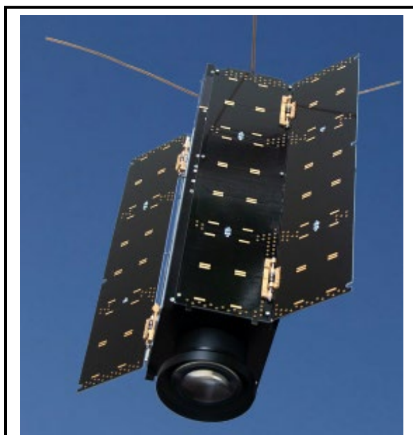
The Hyper-Angular Rainbow Polarimeter (HARP) CubeSat (illustrated above), is demonstrating a new hyper-angular polarimeter that can characterize aerosol and cloud properties. HARP sent back its first images in April 2020. The flight validation is proving that CubeSat-size technology can provide science-quality multi-angle imaging data. In August 2020, HARP was named "SmallSat Mission of the Year" by the American Institute of Aeronautics and Astronautics.
