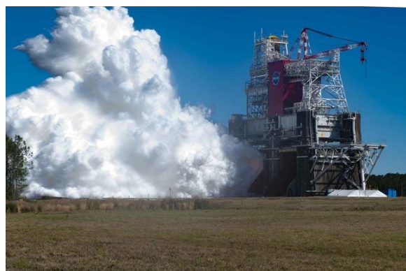
The core stage for the first flight of NASA's Space Launch System rocket is seen in the B-2 Test Stand during a second hot fire test, Thursday, March 18, 2021, at NASA's Stennis Space Center near Bay St. Louis, Mississippi. The four RS-25 engines fired for the full-duration of eight minutes during the test and generated 1.6 million pounds of thrust. The hot fire test is the final stage of the Green Run test series, a comprehensive assessment of the Space Launch System's core stage prior to launching the Artemis I mission.
