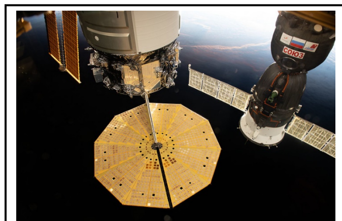
Two spacecraft are pictured docked to the International Space Station. At left, with its prominent cymbal-shaped solar arrays, is Northrop Grumman's Cygnus cargo resupply vehicle. To the right, is the Soyuz MS-17 crew vehicle (October 18, 2020).
