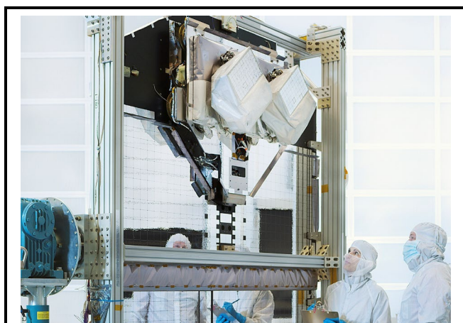
The Laser Communications Relay Demonstration payload, shown here in the clean room at GSFC, will be hosted and flown on a U.S. Space Force technology satellite in June 2021. LCRD will be communicating with two dedicated optical ground stations in California and Hawaii and eventually with a test payload on ISS.
