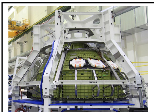
Artemis II crew module's capsule being moved from KSC's Operations and Closeout (O&C) clean room to external work stand for assembling the environmental control and life support and propulsion system.
