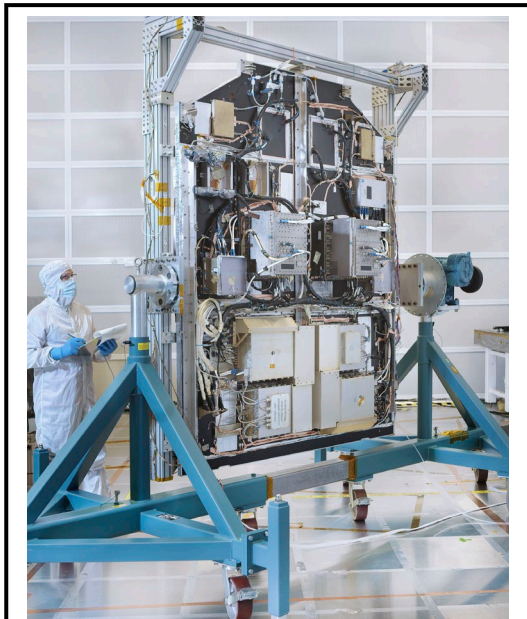
On January 22, 2020, the Laser Communications Relay Demonstration (LCRD) flight payload was delivered to Northrop Grumman's facility in Sterling, Virginia. There the payload will be integrated onto the U.S. Air Force's Space Test Program Satellite 6 (STPSat-6) and prepared for launch. LCRD will be NASA's first end-to-end optical relay, sending and receiving data from missions in space to mission control on Earth. This image shows the LCRD space switching unit, which will enable digital communications from space to ground.
