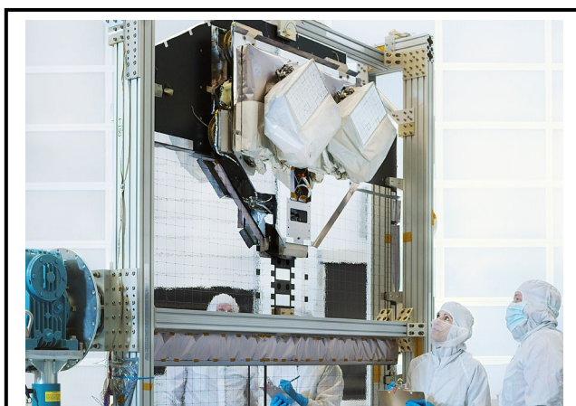
The Laser Communications Relay Demonstration (LCRD) flight payload (pictured above) was delivered to Northrop Grumman's facility in Sterling, Virginia. There, the payload was integrated onto the U.S. Space Force's Space Test Program Satellite 6 (STPSat-6) in preparation for launch. LCRD will be NASA's first end-to-end optical relay, sending and receiving data from missions in space to mission control on Earth.
