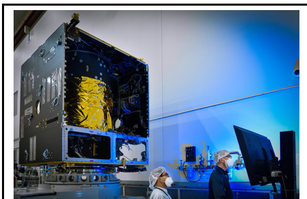
Assembly of the Psyche spacecraft chassis at the Maxar facilities in Palo Alto, CA. The team powered on the Psyche spacecraft for the first time in the factory and began reading telemetry.
