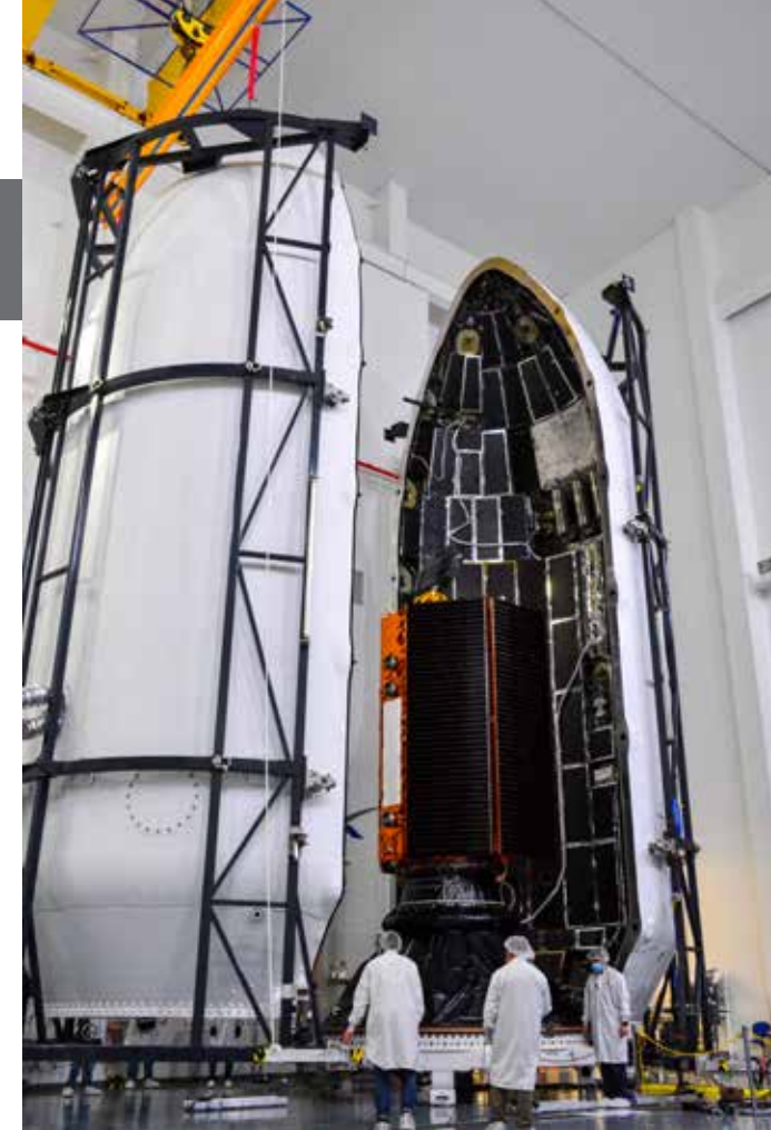
The U.S.-European Sentinel-6 Michael Freilich ocean-monitoring satellite is encapsulated in the SpaceX Falcon 9 rocket's payload fairing on Nov. 3, 2020, inside SpaceX's Payload Processing Facility at Vandenberg Air Force Base (VAFB) in California. Credit: NASA/Randy Beaudoin
