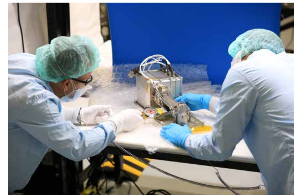
Engineers and technicians at NASA's Kennedy Space Center in Florida install the radiator for the Mass Spectrometer Observing Lunar Operations (MSolo) instrument inside the Space Station Processing Facility on Sept. 25, 2020. Credit: NASA/Glenn Benson
