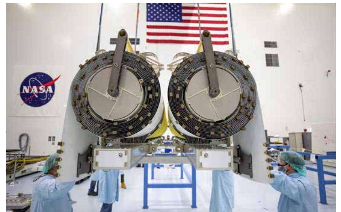
NASA and Boeing workers help position solar arrays bound for the International Space Station onto flight support equipment inside the high bay of the Space Station Processing Facility at NASA's Kennedy Space Center in Florida on April 2, 2021. Credit: NASA/Frank Michaux
