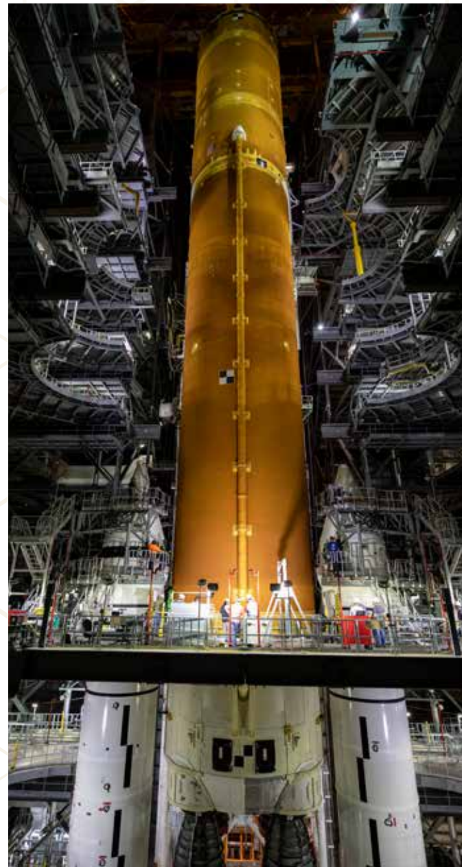
Teams with NASA's Exploration Ground Systems and contractor Jacobs lower the Space Launch System (SLS) core stage – the largest part of the rocket – onto the mobile launcher, in between the twin solid rocket boosters, inside High Bay 3 of the Vehicle Assembly Building at NASA's Kennedy Space Center in Florida on June 12, 2021. Credit: NASA/Cory Huston
