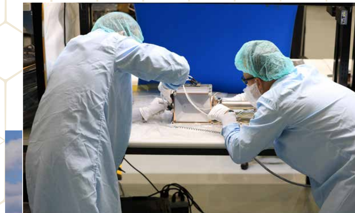
Engineers and technicians install the radiator for the Mass Spectrometer Observing Lunar Operations (MSolo). Credit: NASA/Glenn Benson
