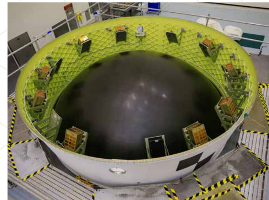
Small satellites, called CubeSats, are shown secured inside NASA's Orion stage adapter at NASA's Kennedy Space Center in Florida on Aug. 5, 2021. Credit: NASA/Cory Huston
