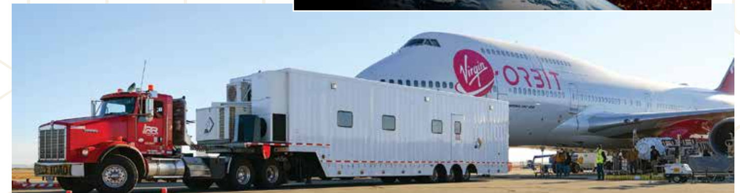
Virgin Orbit's mobile payload trailer pulls up next to the carrier aircraft Cosmic Girl to integrate the encapsulated payload assembly, carrying several NASA-sponsored small satellites for the company's Launch Demo 2 mission on Nov. 30, 2020. Credit: Virgin Orbit/Greg Robinson
