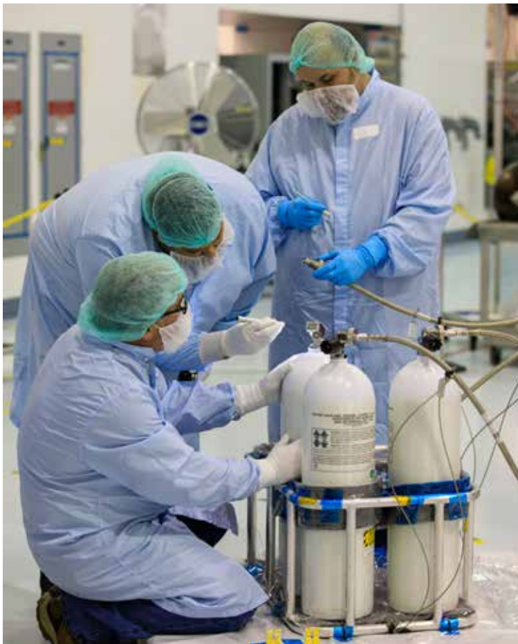
Inside the Space Station Processing Facility at NASA's Kennedy Space Center in Florida on June 25, 2021, commercial off-the-shelf air tanks – normally used by divers – are filled with breathing air for use on the International Space Station. Credit: NASA/Kim Shiflett
