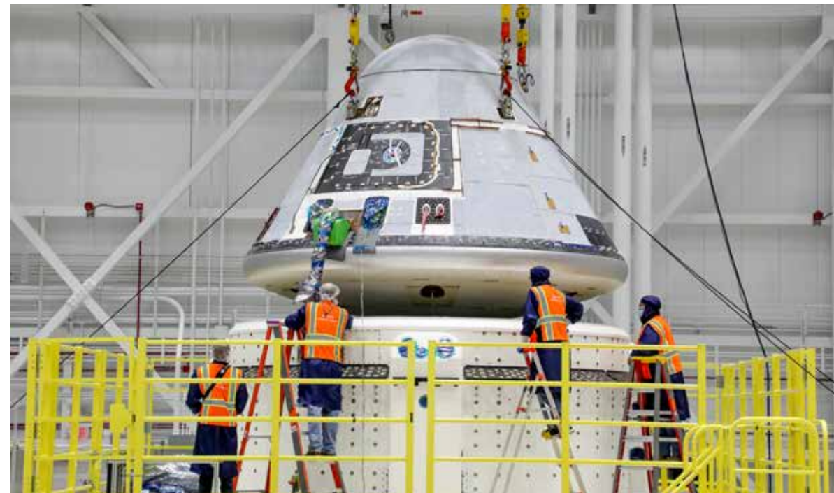
Technicians observe Boeing's Starliner crew module being placed on top of the service module in the Commercial Crew and Cargo Processing Facility at NASA's Kennedy Space Center in Florida on Jan. 14, 2021, in preparation for NASA and Boeing's OFT-2 mission. Credit: Boeing/John Proferes
