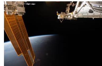
The Roll-Out Solar Array (ROSA) is a new, more compact solar panel that will snap open in space, a favorable design over the rigid solar panels currently in use, pictured above. Credits: NASA
