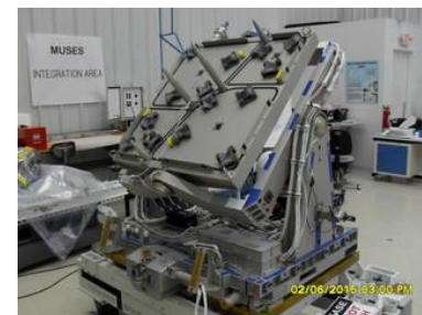
MUSES hosts earth-viewing tools such as high-resolution digital cameras and hyperspectral imagers and provides precision pointing and other accommodations. It hosts up to four instruments at the same time, and offers the ability to change, upgrade, and robotically service those instruments. Credit: Teledyne Brown Engineering
