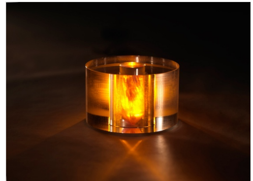
The room-temperature maser relies on a crystal of organic molecules excited with an optical laser.
