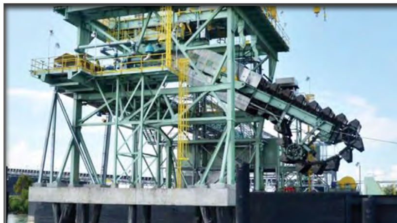
Figure 4-3. Continuous bucket unloading system for barges
