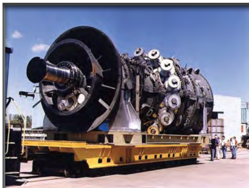
Figure 7-2. Large gas turbine prepared for shipment; combustors, pre-fabricated manifolds, and control skids will be shipped separately
