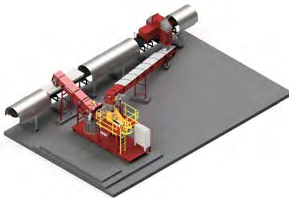
Figure 4-5. A swing-arm/cross belt sampler as part of a sampling system
