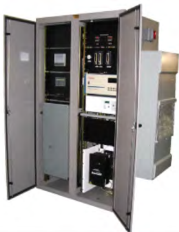
Figure 13-10. Online laser fuel analyzer
