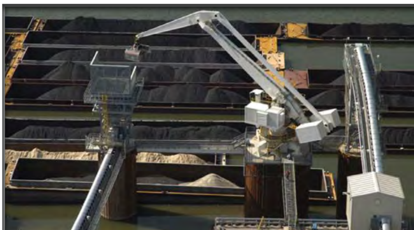
Figure 4-2. A clamshell, or balance crane, unloader for barges
