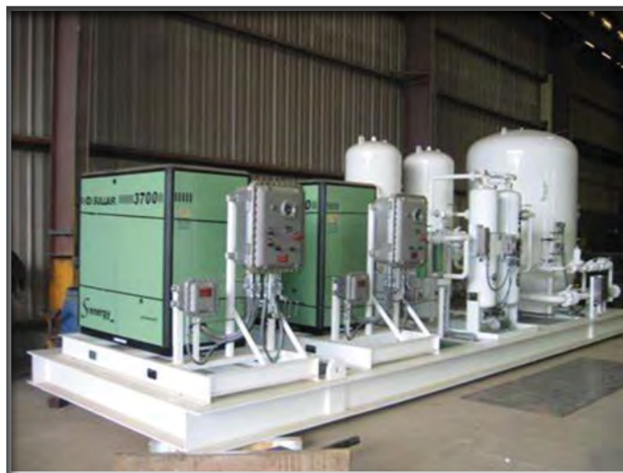
Figure 13-4. Skid-mounted compressed air system
