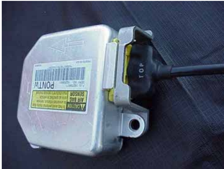
Figure 4-3. GM EDR shown connected to Vetronix CDR download cable [Kerr 2002, used with permission of the Vetronix Corporation]
