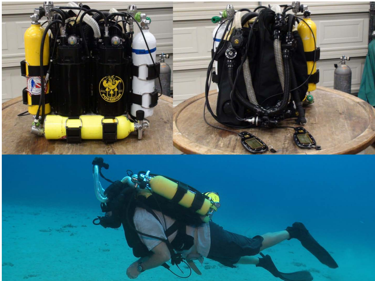
Figure 7. Prototype dual-loop rebreather system designed and tested by the author.
