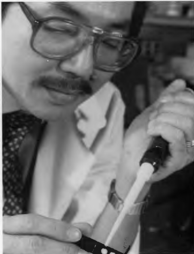
Tuan Vo-Dinh demonstrates the simplified PCB spot test. The newly developed test uses strips of chemically treated paper that glow when exposed to ultraviolet light if the liquid sample coating the strip is contaminated with PCBs.
