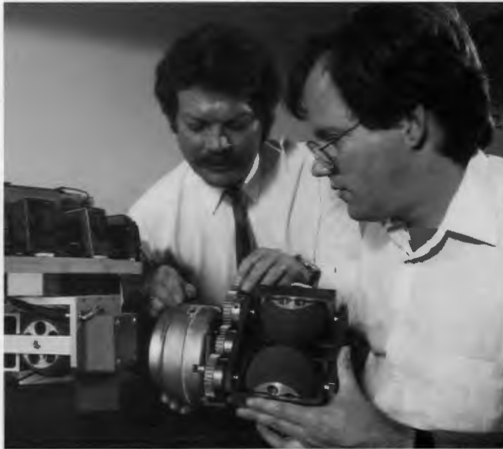
Francois Pin and Stephen Killough demonstrate the Omnidirectional Holonomic Platform, which promises big improvements for wheeled devices such as motorized wheelchairs, factory and plant equipment, robots, and even household vacuum cleaners. The ORNL device can do what conventional wheeled vehicles are unable to do—move in all directions from a starting position while spinning.
