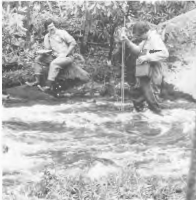
Glenn Cada and Jim Loar, both of ORNL's Environmental Sciences Division, measure the discharge of Bradley Creek in North Carolina as part of a study of trout-habitat and stream-flow relationships in 1983 for the DOE hydropower program. Photograph by Mike Sale
