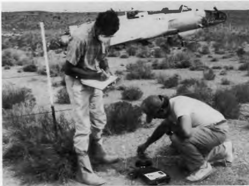
Dick Gammage records Kevin Meyer's readings of electret detector voltages from an electrometer during field studies at the Nevada Test Site. The plastic detectors (the small black cylinders in the photograph) measure alpha emissions from plutonium-contaminated soil. The work is being done as part of a CRADA with Rad Elec, Inc.
