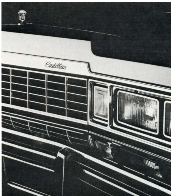
Figure 3 - Grille shows beauty and practicality achieved by plating on molded plastic. Electroless copper is used as conductive base because it permits long life in corrosive environments.
