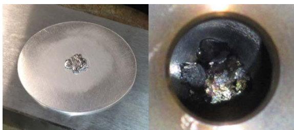
Fig. 1: ^{92}\text{Mo} powder was melted, rolled, and afterwards pressed onto an Al backing. Photo of the target before (left) and after (right) irradiation.
