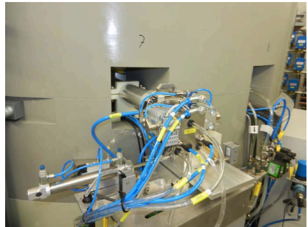
Fig. 3: The solid target station for the production of radionuclides.
