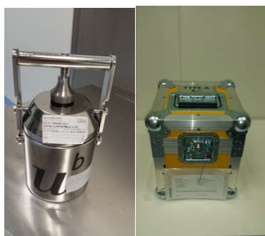
Fig. 2: Transportation of DCB-UNIBE [ ^{68}\text{Ga} ]-DOTATATE in the lead container and type A box.
