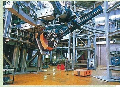
ITER In-vessel Remote Maintenance Device for blanket
