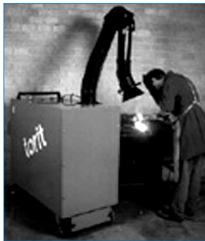
Figure 2.10 Local exhaust ventilation system for welding and soldering purposes (Source: www.dce.co.uk )
