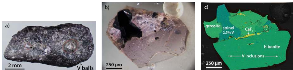
FIGURE 4. Hibonite-grossite aggregates. (a) Large grain of hibonite-grossite aggregate with millimeter-size spheres of native V ( V^0 ). (b) Transmitted-light photo of the transparent specimen, enclosing black spinel grain and rods of V^0 . (c) Phase map of b showing paragenesis of aggregates. Comparison of b and c shows that each tiny V^0 inclusion represents the end of a long rod or dendrite branch. (Color online.)
