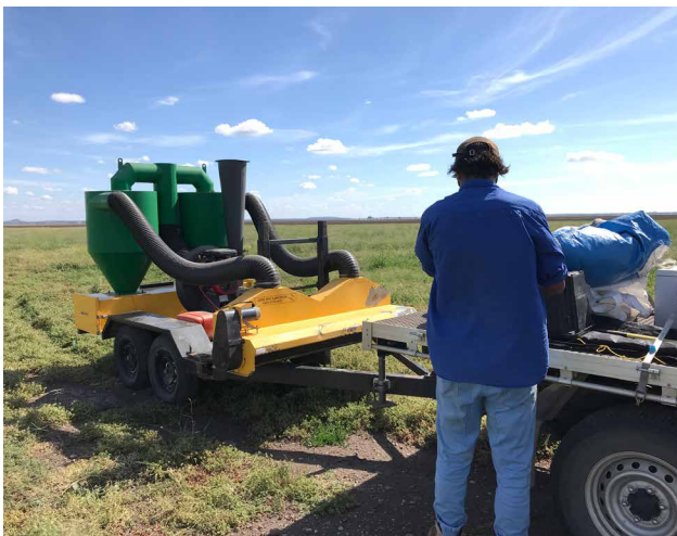
'Rosevale Reaper' grass seed harvester, which is towed behind a ute in an offset position. Similar equipment is suitable for small, odd-shaped or uneven paddocks.
