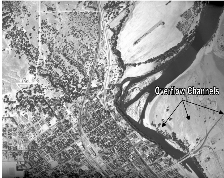
Image Comparison 1a. Red Bluff and the Sacramento River in 1938 (top) and 2004 (bottom). Note the two large islands at the bend of the river and the large overflow area to the east of Red Bluff in 1938 and compare the 2004 situation. These changes are likely due to Shasta Dam's moderation of river flows during floods.
