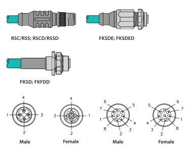
The 4-pin M8, rated for IP67, is also available for use in Industrial Ethernet applications. The smaller size of the M8 allows users to bring Industrial Ethernet into applications with very limited space. It is available with the shield tied to the coupling nut, as required by the EtherCAT network protocol. The 4-pin configuration is suitable for 2-pair Industrial Ethernet cables.
