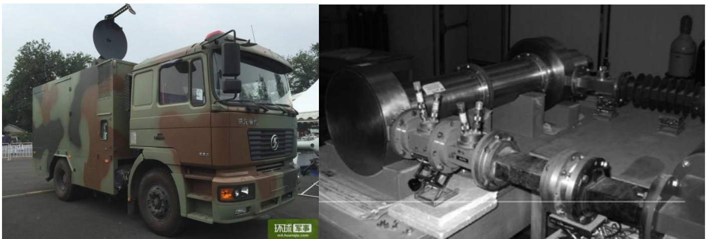
At the 2014 Zhuhai Airshow (left) China's POLY company revealed their WB-1 "active denial" microwave weapon, which can repel unruly crowds out to 80 meters. Images of a possible experimental microwave weapon component (right) appeared on Chinese web pages in early 2017, coinciding with reports late January 2017 Chinese press reports of an award for an engineer with the Northwest Institute of Nuclear Technology, for having developed microwave weapons that could defend ships from attacking missiles. Source: Huanqiu and Chinese Internet
