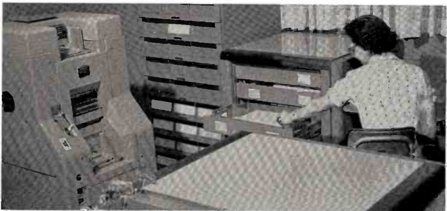
BELOW: This view shows the alphabetical punch that accommodates variable or temporary information by punching holes in cards, and (at left) the collator that assembles several sets of cards into one set in numerical sequence. Checking the file is Olga Slota.
