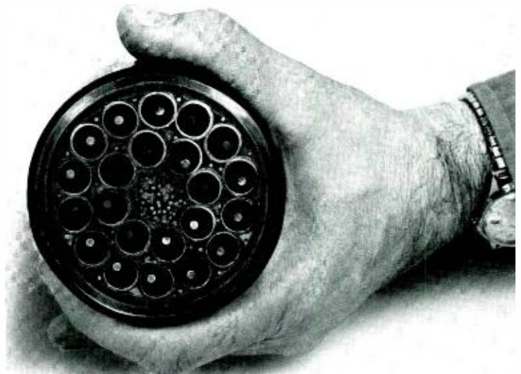
Cross-section view of the 22-tube coaxial cable, part of the L5 transmission system. This super-capacity transmission facility can carry 108,000 simultaneous telephone conversations—more than three times the capacity of previous cable systems.
