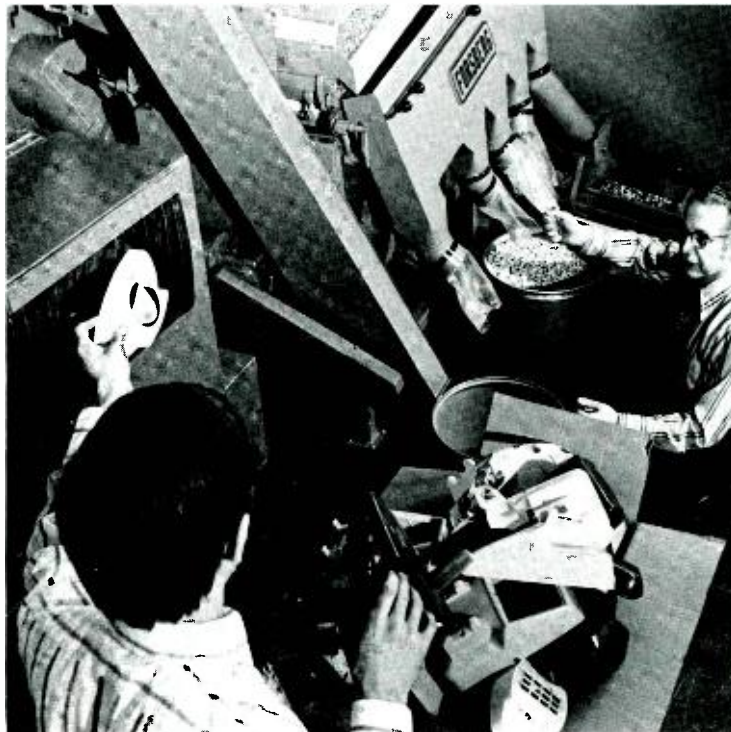
In 1974 Bell Labs scientists, working with Western Electric engineers, developed a way to recycle plastics from discarded telephone housings and handsets. The discarded housings are ground up into pellets which are then fed into a machine that separates the plastic from the dust, paper, small metal clips, and other materials present in the scrap. At left, Jerry Hardiman feeds housings into the grinding machine while Philip Hubbauer checks the resulting pellets.
