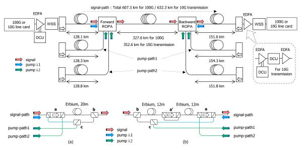
Fig. 1: (TOP) Experimental setup for single 100G/10G channel unrepeatered transmission using two additional ROPA pumping fibers. Insert (dashed box) shows the equipment used for 10G transmission. (BOTTOM) Configurations of (a) forward ROPA, (b) backward ROPA. a, a' : hybrid filter (consists of sig/pump Mux, isolator, and sig/pump Mux), b : sig/pump Mux, c : pump  $\lambda 1/\lambda 2$  Mux.
